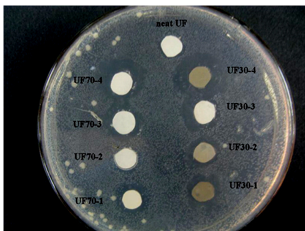
Fig. 12. Inhibition zone areas of different fabricated membranes containing various amount of Ag [151].
